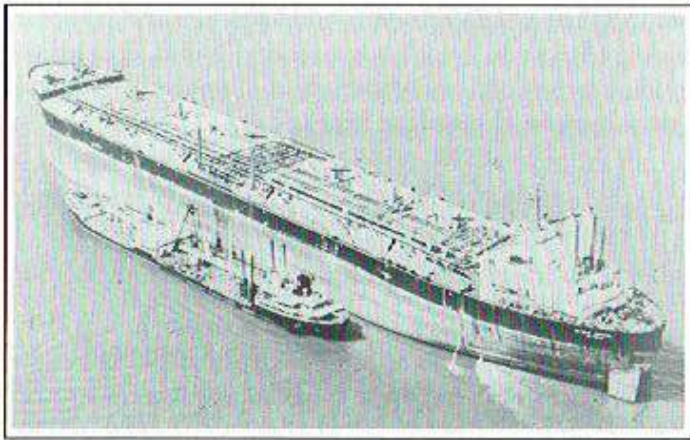
Dwarfing a T-2 tanker (16,600 DWT), the S/S UNIVERSE IRELAND had an 81' draft. Ludwig's success in constructing and operating the 327,000 DWT tankers induced a worldwide mass-ordering of supertankers during the 1970s.
