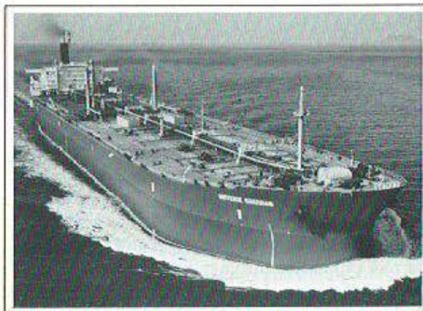
One of eleven vessels of 270,000 DWT constructed for Ludwig in the 1970s, the S/S UNIVERSE GUARDIAN had an increased beam and shallower draft. This new design provided access to more ports and greater flexibility in operation.
