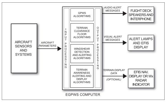
Figure 2-- Enhanced GPWS (EGPWS) BLOCK DIAGRAM.
