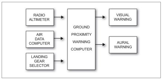
Figure 1 -- 1967 GPWS Computer System Block Diagram.
