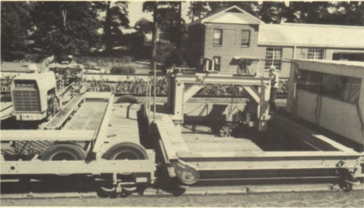
Soil bin research equipment for studying the behavior of full-scale tillage tools.
