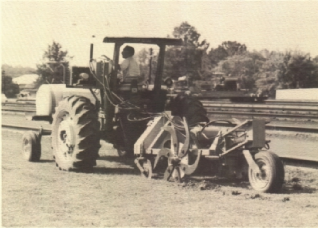
The NSDL power-take-off driven rotary chisel mounted on an instrumented-tractor to study tillage effectiveness and energy efficiency.
