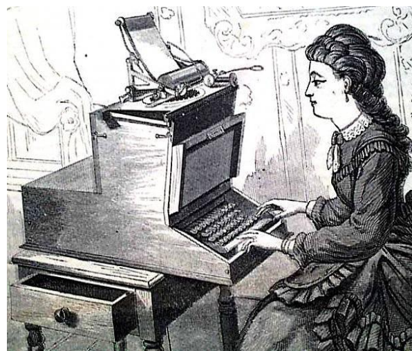
A typist operating a Sholes & Glidden Type Writer, as depicted in an 1872 article in Scientific American .
