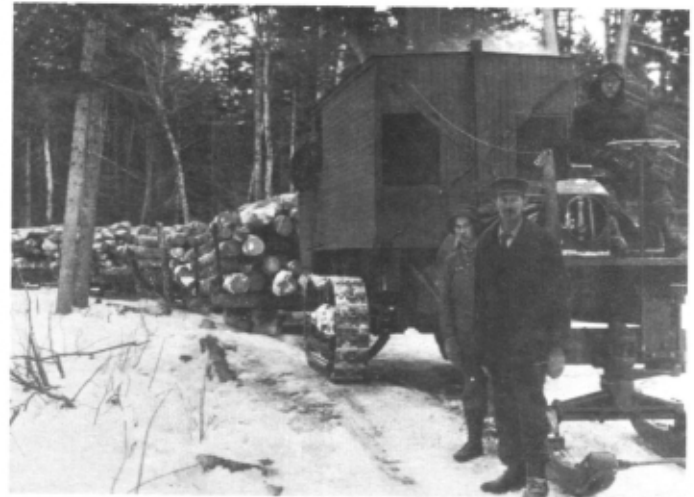
A typical log hauler crew consisted of an engineer, fireman, conductor, and the steerer. The conductor, riding close to the rear, communicated with the cab by a bell rope which ran along the sled stakes.
