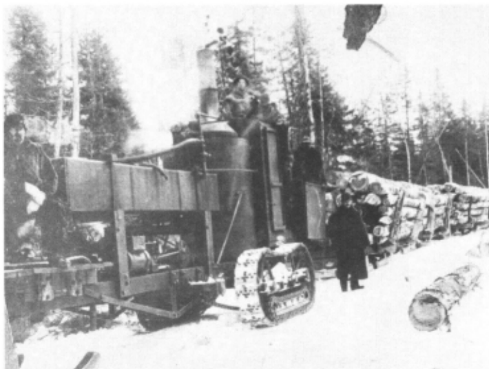
Early type of Lombard Steam Log Hauler with upright boiler and engine.
