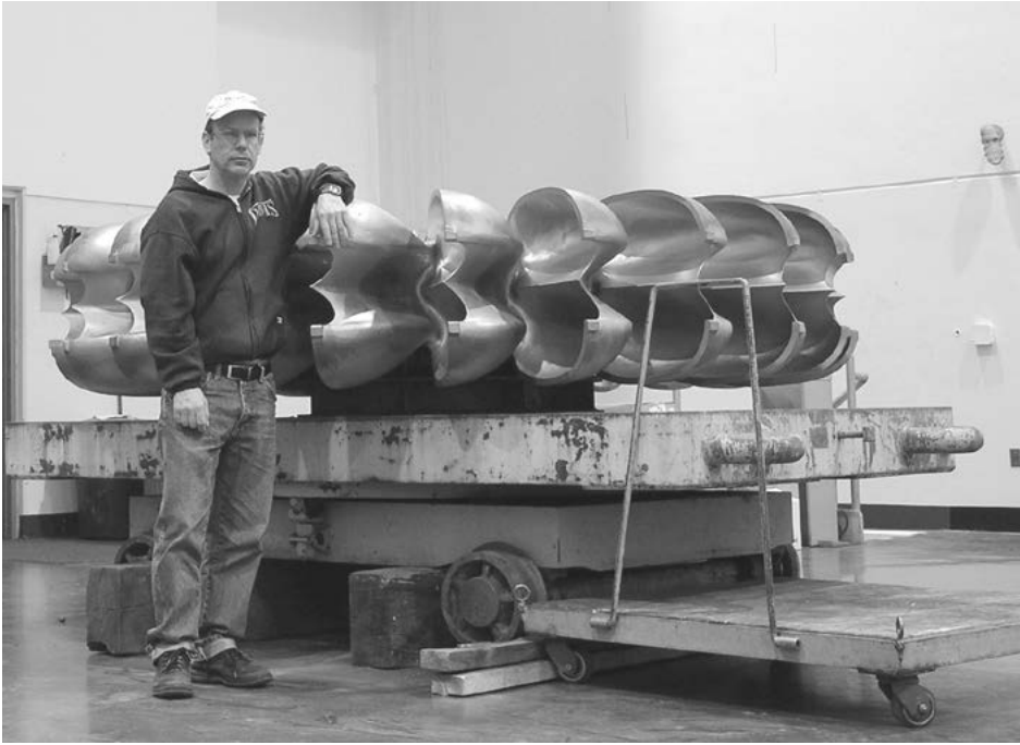
Figure 2. Matthew Gass [7] , of California's Hetch Hetchy Water and Power, inspecting a 47 MW, 327 rpm, 1280 ft net head Pelton wheel at the Kirkwood Powerhouse (located about 125 miles south of the goldfields where Pelton invented the wheel in 1880).
