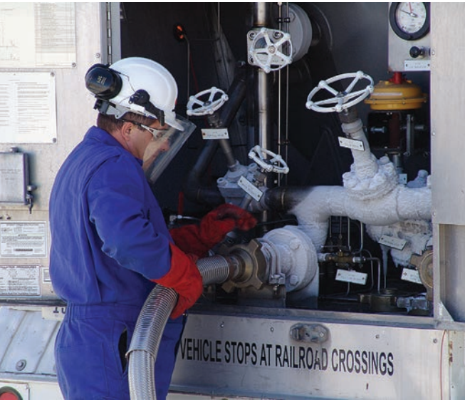
A driver wears insulated gloves and a face shield as he transfers LNG from a terminal to a tanker truck.
