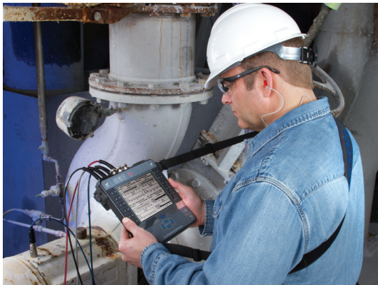
In smaller factories, technicians typically monitor bearings by using portable vibration monitors.
