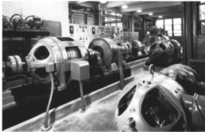
A portion of the equipment that controls the speed and pressure in the Water Tunnel
